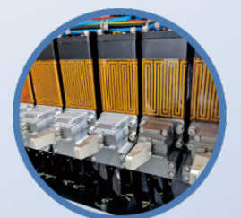
Build-in heaters & Negative pressure
